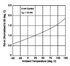
Figure 3. Typical Normalized On-Resistance
